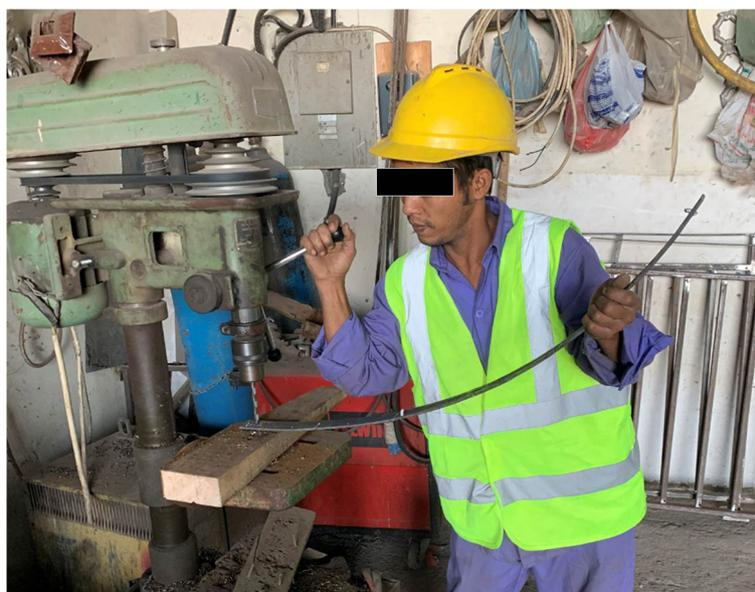
**Fig. 1** A worker at a small-scale industrial enterprise at the main industrial area of Al-Ain City drilling a hole in a metallic bar over a wood block using a large electrical drill without personal protective eyewear (The worker gave his written consent to use his picture for publication)
