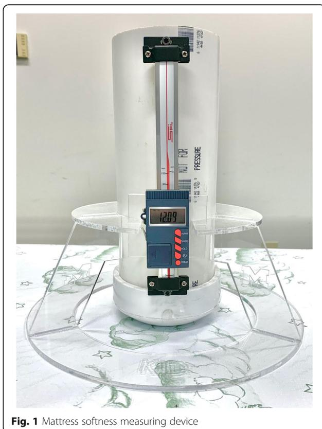
**Fig. 1** Mattress softness measuring device
